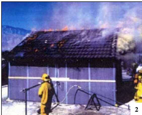
Test building with a stone-coated metal roof during a simulated attic fire.
